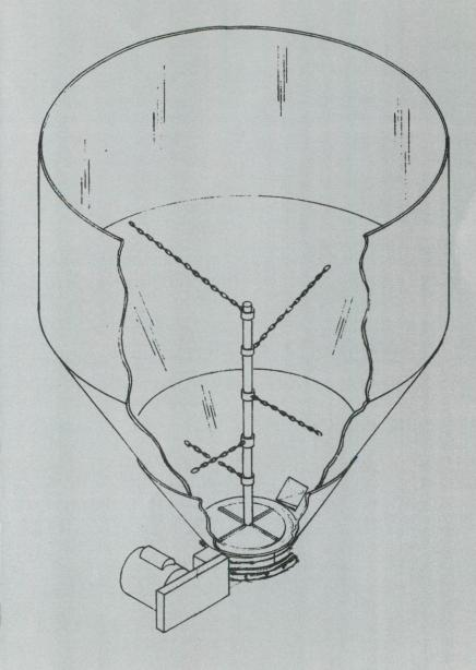
**BULK BIN AGITATOR UNLOADER**For Center Draw Bulk Bins
